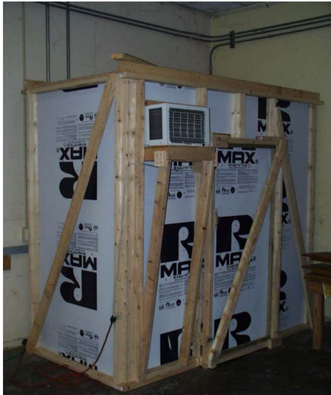
Figure 3.8 Environmental chamber used in controlled pilot tests
